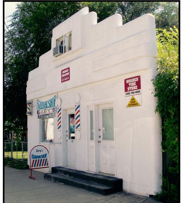
Over the years, Hughes closed in some of the back sections, beefed up the trusses, installed flooring in the upper level in order to store tires, and insulated the building. The original building only had sawdust shavings in the walls for insulation.
